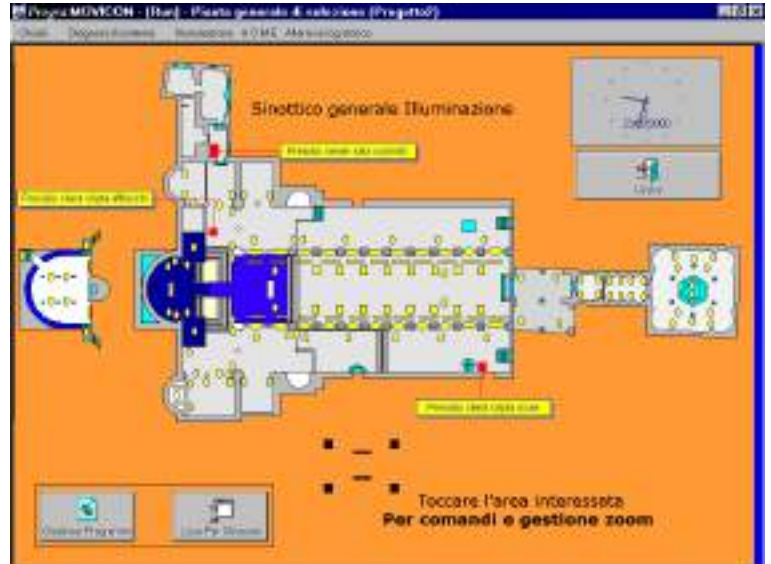
One of the Movicon's screens that manage the supervision of the historical cathedral Basilica of Aquileia.
