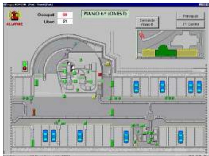
One of the screens displayed on a car park attendant control terminal.
