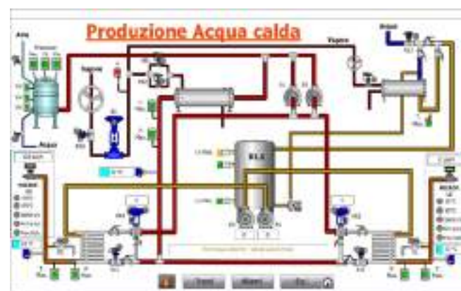
Hot water production monitoring and control
