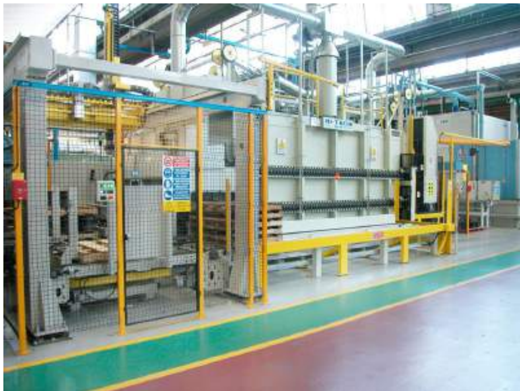
The final Palletization stage in the new roller tempering production line process belonging to the Italian manufacturers of track loader components.
