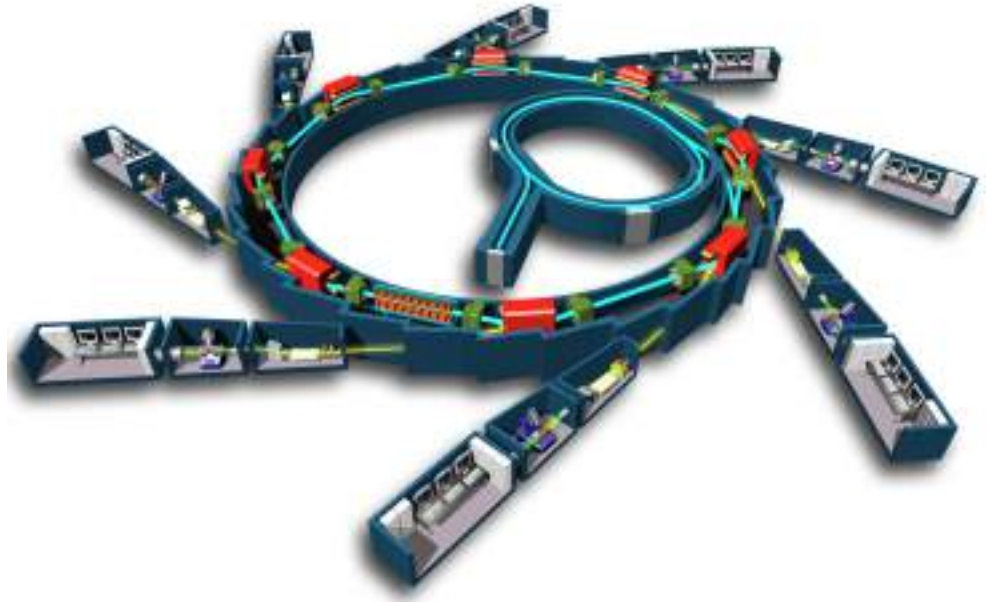
A generic scheme of the circular rotating particle accelerator whose magnetic field (needed for bending the trajectory of the particles) and the variable electric field (which accelerates the particles) are synchronized with the beam of particles.
