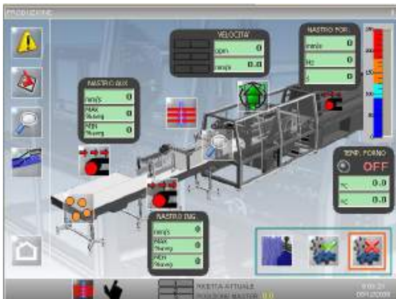
The Movicon main screen showing the Kosme Flypack machine.
