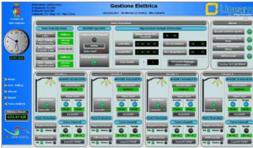
3. Screen of one of the workstations configured with the astronomical clock status and settings as well as the various options.
