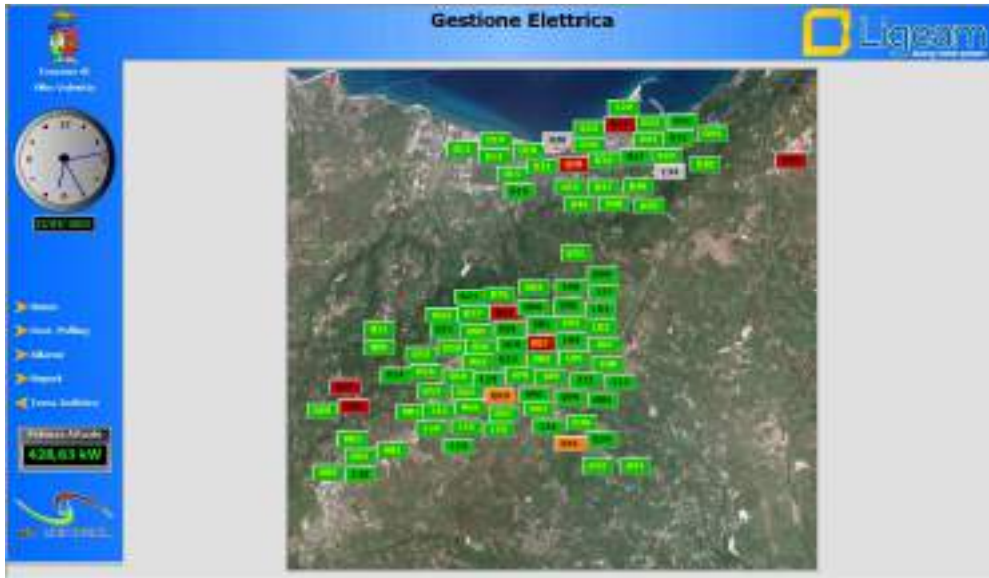
1. The Movicon Home Page showing electrical plant management localization
