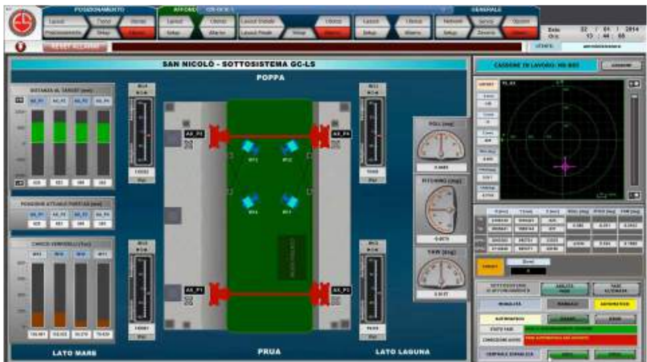
4. Movicon threshold caisson display screen
