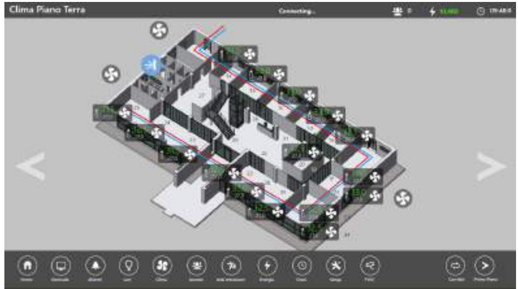
The air conditioning system is connected to the Movicon.NExT supervisor via BacNet/IP bus.
