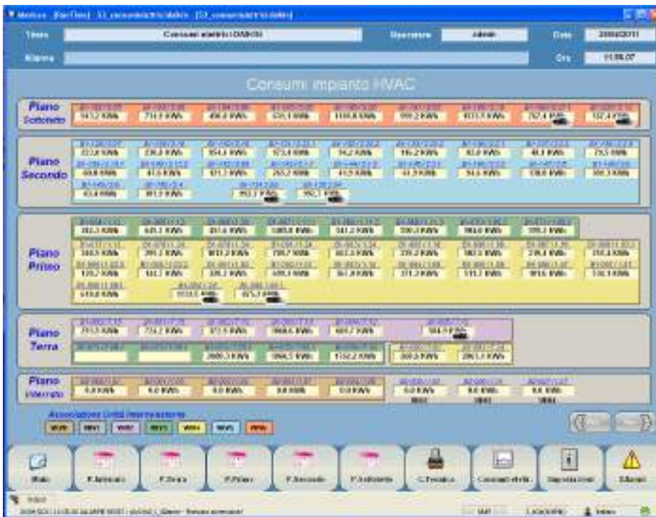
Figure 4 – Screen displaying HVAC system consumptions
