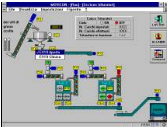
A Movicon dropdown window containing manual plant actuator commands
