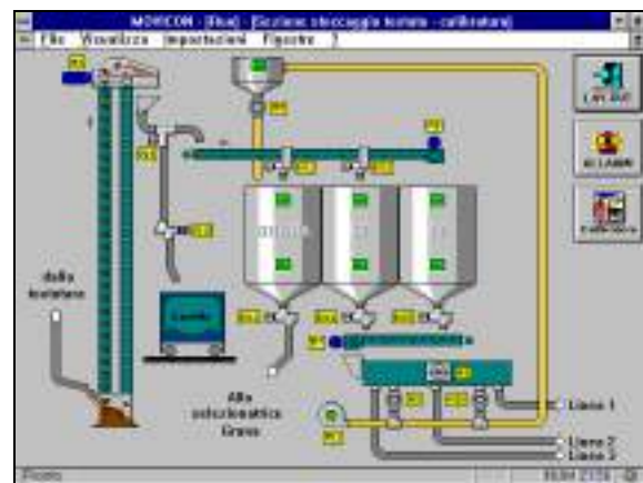
A Movicon dropdown window containing manual plant actuator commands
