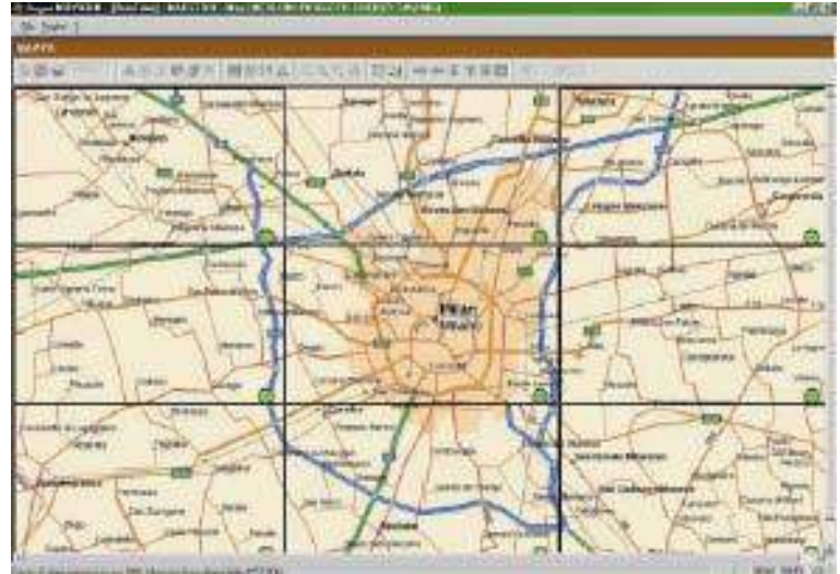
Figure 2 – This shows interaction between animated map, anagraphical data and telecontrol. A green light, on the bottom right of each square on the map, means that there have been no alarm occurrences in that zone as yet.
