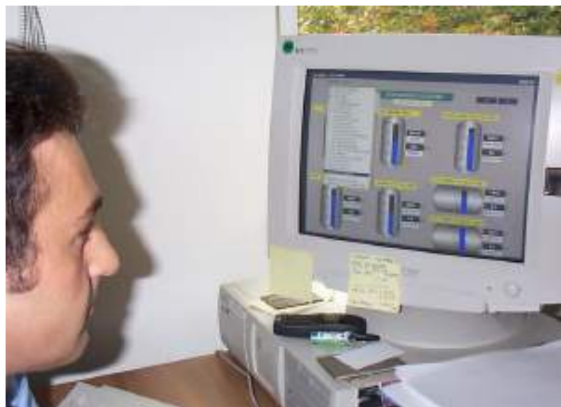
A telemetric station based on Movicon Web Client, installed in the offices of the engineering division of Monza (MI). Thanks to Web Client technology, the office is linked to the Movicon server to which the data of the telemetric system are sent.
