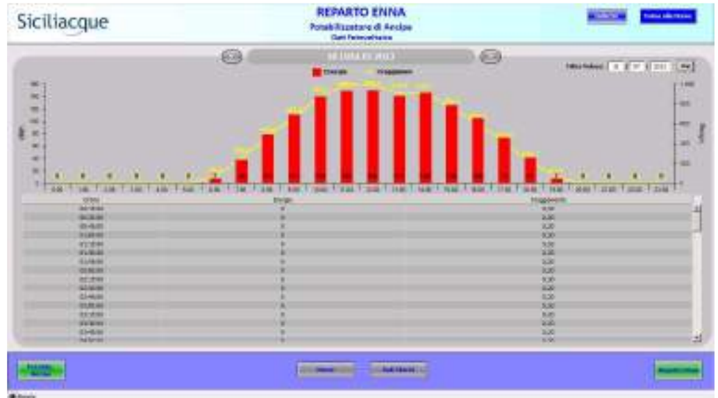
4. Photovoltaic data of the Ancipa water purification system. Energy and irrigation data recording.
