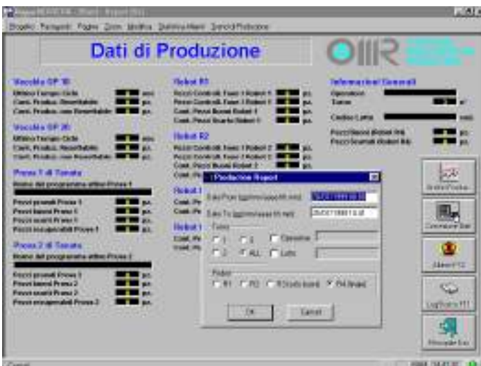
This page reports production data in realtime. The operator can use this page to get statistical production analysis by specifying the required information. Movicon creates statistic reports and production chart graphics.
