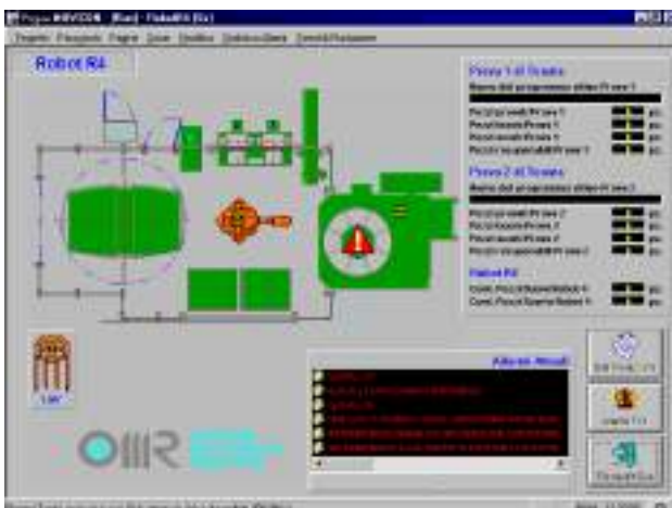
A detailed Movicon screen page, where the operator can manage and control the production line and each of its components.
