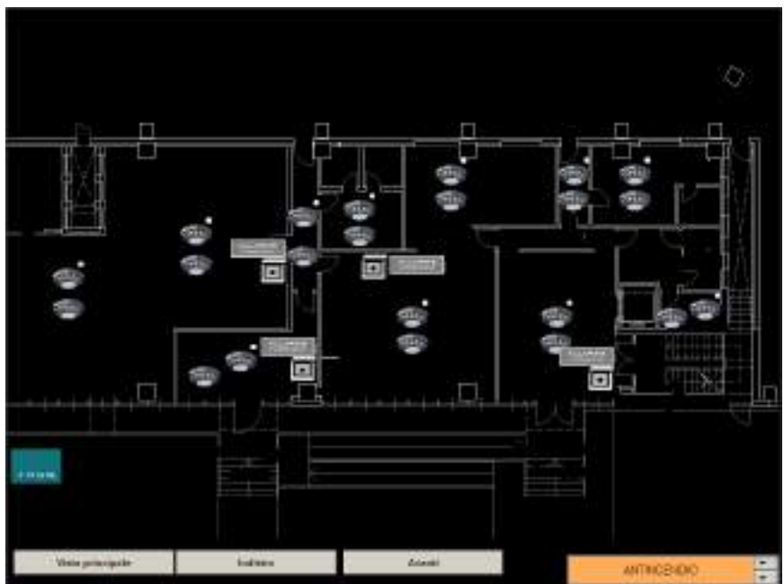
One of the integrated supervision system screen pages. Visualization of the whole system is completely accessible using web architecture.
